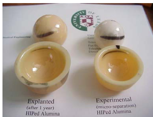
Figure 1. "Stripe" wear of HIPed alumina components
